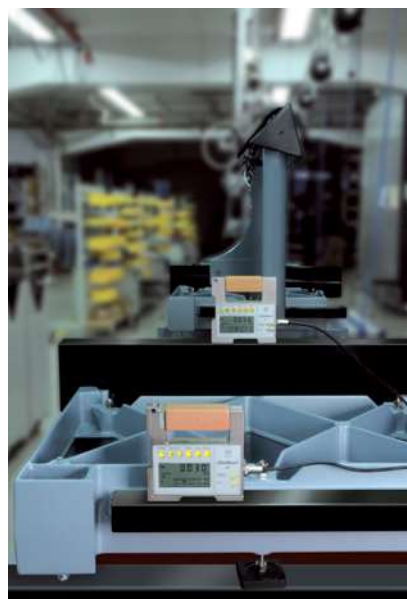
When 2 CLINOBEVEL 2 are connected, one of the instruments becomes the reference
